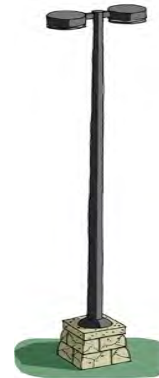
Double luminaire “hatbox” parking lot light on limestone patterned concrete base.
